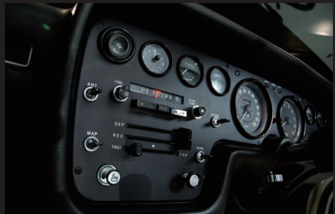
The center console is arranged with the radio on the upper part and the heater controls on the lower part. The triple gauge cluster features, from left to right, a clock, a fuel gauge, and an ammeter.
