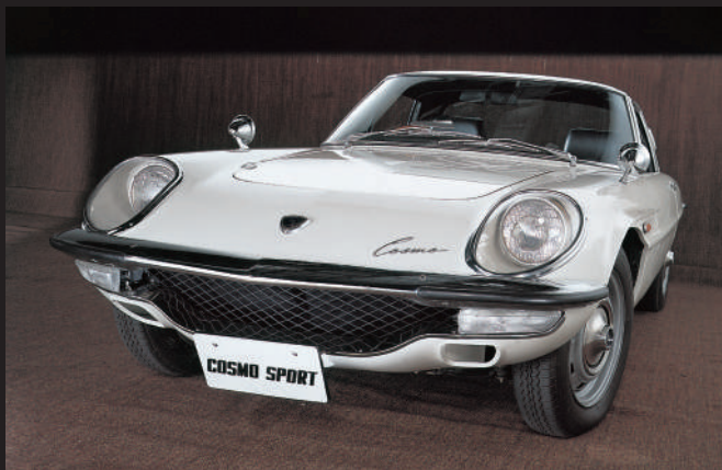
This is the later model. Unlike the earlier version shown on the previous page, the air intake below the bumper has been enlarged.
