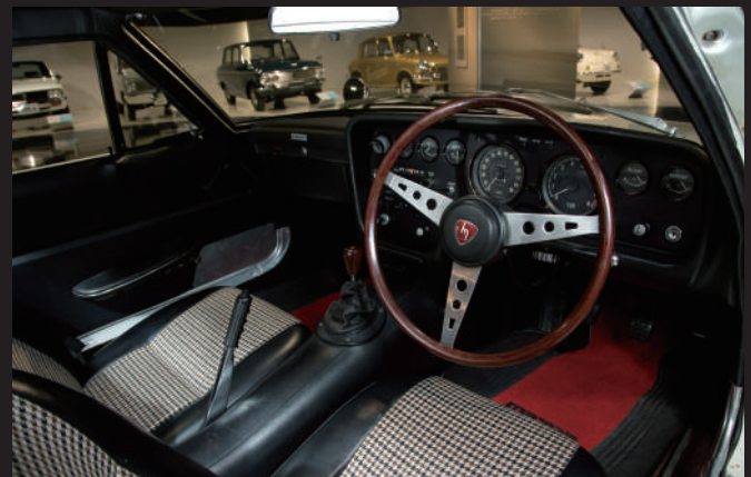
The dashboard area of the Cosmo Sport. By adjusting the dial located on the right side of the steering column, the steering wheel can be moved forward or backward.
